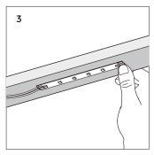
Clean the environment part to be attached with a cloth, as shown in Figure 1, and then tear off the 3M tape on the back of the light belt, and finally stick the light belt on the clean place.
